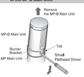
After disengaging the tabs on both sides, lift the MP-B Main Unit upward to remove.
